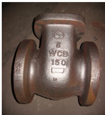
Figure 4: A sample of cast GTV valve body (photo)
