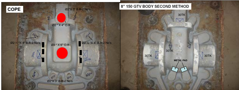
Figure 2: Pattern of Mould Design two ( M_2 ) for GTV valve body (photo)
