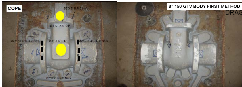
Figure 1: Pattern of Mould Design one ( M_1 ) for GTV valve body (photo)
