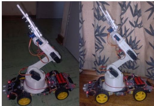
Figure 3: Prototype of the remote-controlled assistive robotic arm
