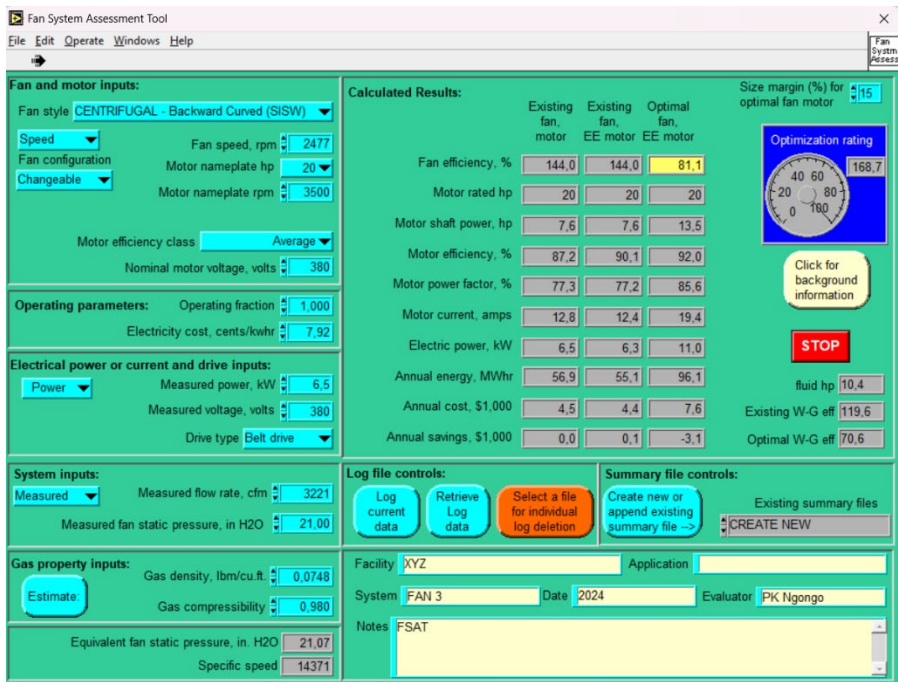
Figure 6: Fan 3 system assessment
