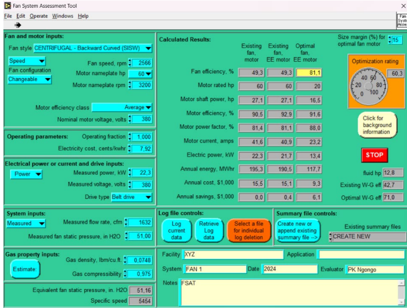
Figure 4: Fan 1 system assessment
