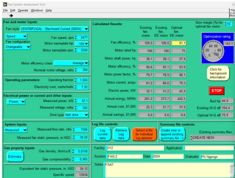
Figure 5: Fan 2 system assessment
