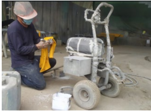
Figure 9: Procedure for changing parts of painting equipment
