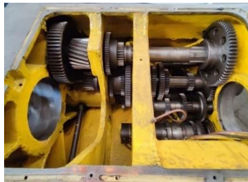
Figure 2: Internal diagram of remanufactured spindle box
