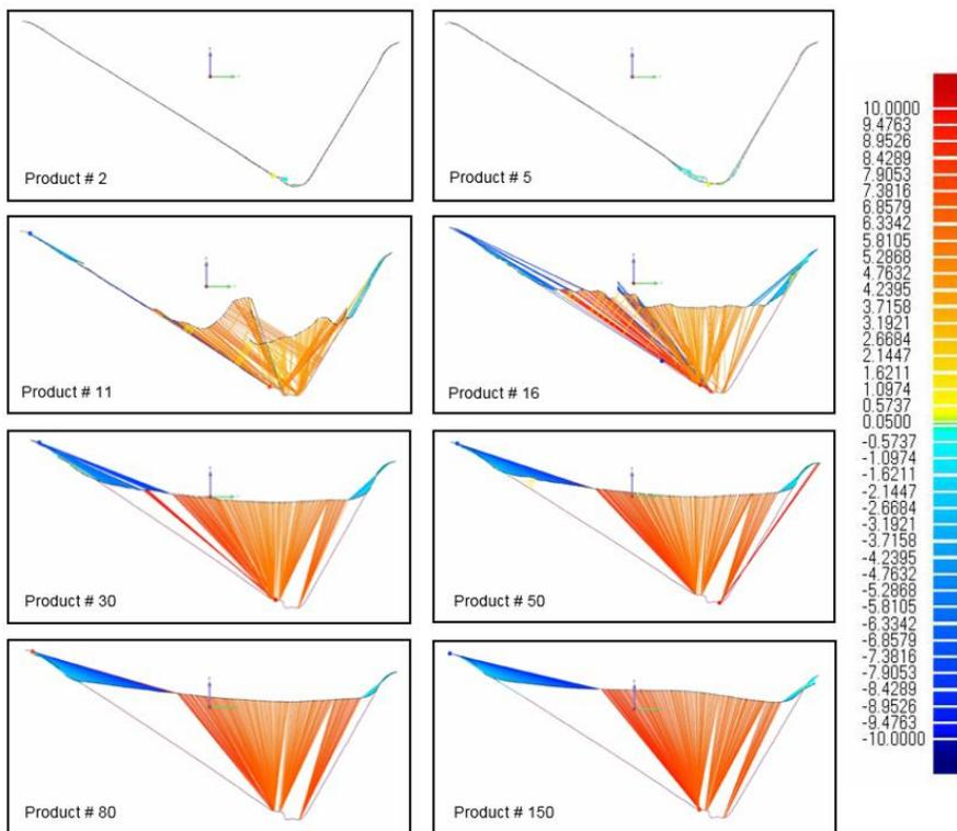
Figure 13: Graphical representation of the wear progression of a geometrical feature from the fixed half of the Alumide<sup>®</sup> insert from an IM trial with PA 6 material (see online version for colour)
