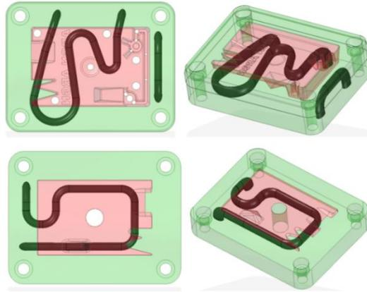
**Figure 2: Layout of the oval conformal cooling channels avoiding insert features such as screw and ejector pin holes**
