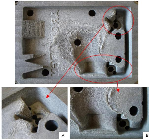
Figure 12: Moving half of the Alumide<sup>®</sup> insert after 150 IM cycles using PA 6. Figures A and B are enlargements of the circled regions of the insert
