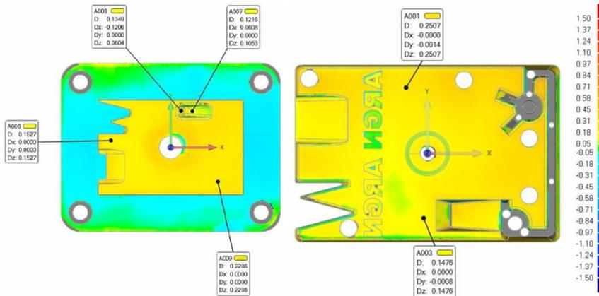
Figure 5: Scan results of the Alumide<sup>®</sup> inserts after 200 IM cycles using PP (see online version for colour)
