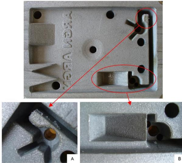
Figure 4: Moving half of the Alumide<sup>®</sup> insert after 200 IM cycles using PP. Figures A and B are enlargements of the circled regions of the insert
