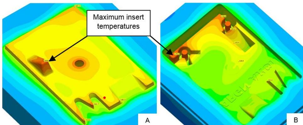
**Figure 3: Insert features where the maximum temperatures occur for the fixed (A) and moving (B) Alumide® inserts after the 20<sup>th</sup> IM cycle, according to SIGMASOFT® virtual moulding software (see online version for colour)**
