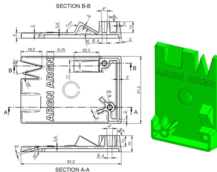
**Figure 1: Dimensions and CAD model of the different geometrical features included in the test product to be produced using Alumide® inserts**
