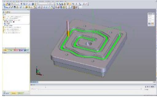
**Figure 10: NC toolpaths programmed using EdgeCam 2014 R1**
