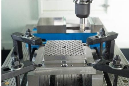
**Figure 12: CNC machining of conventional manufactured insert**
