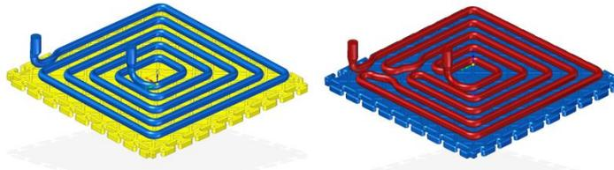
**Figure 13: Spiral and meander conformal cooling design**
