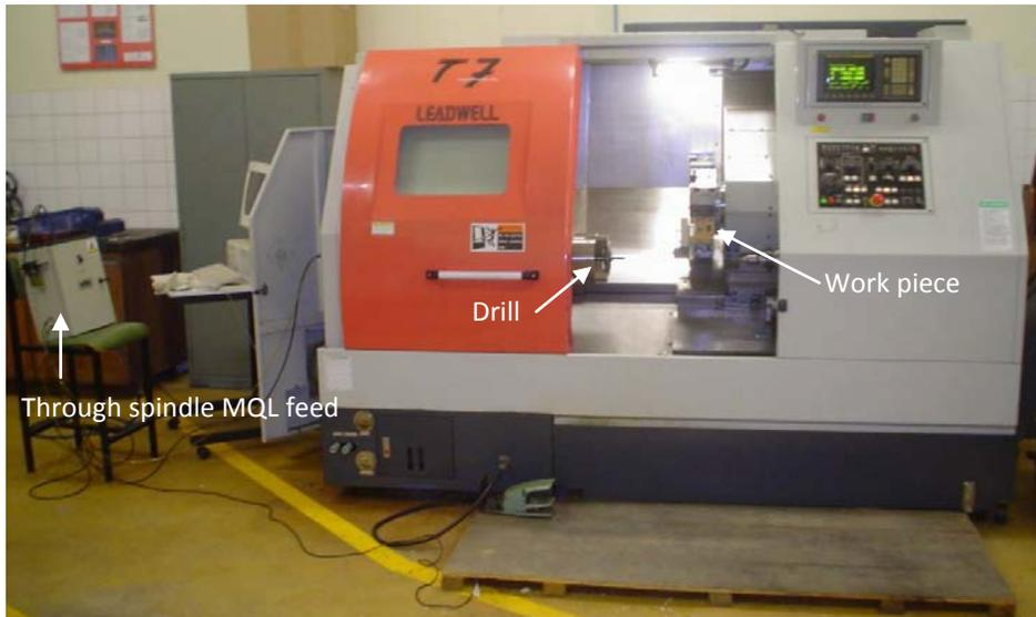
Figure 4: Experiment to simulate horizontal drilling
