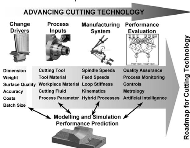
Figure 1: Primary aspects associated with advancing cutting technology [1]
