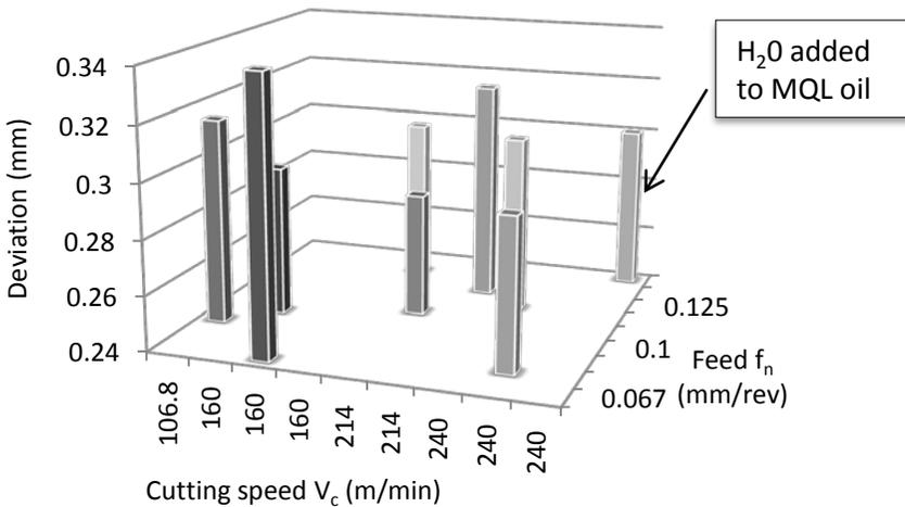
Figure 9: Hole deviations for the indexable step and chamfer drill experiments
