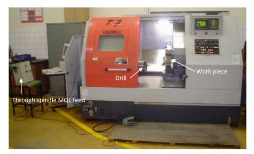
Figure 4: Experiment to simulate horizontal drilling
