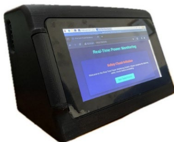
Figure 3: AI-powered advanced energy monitoring device integrating precision sensors and real-time data processing for efficient home management
