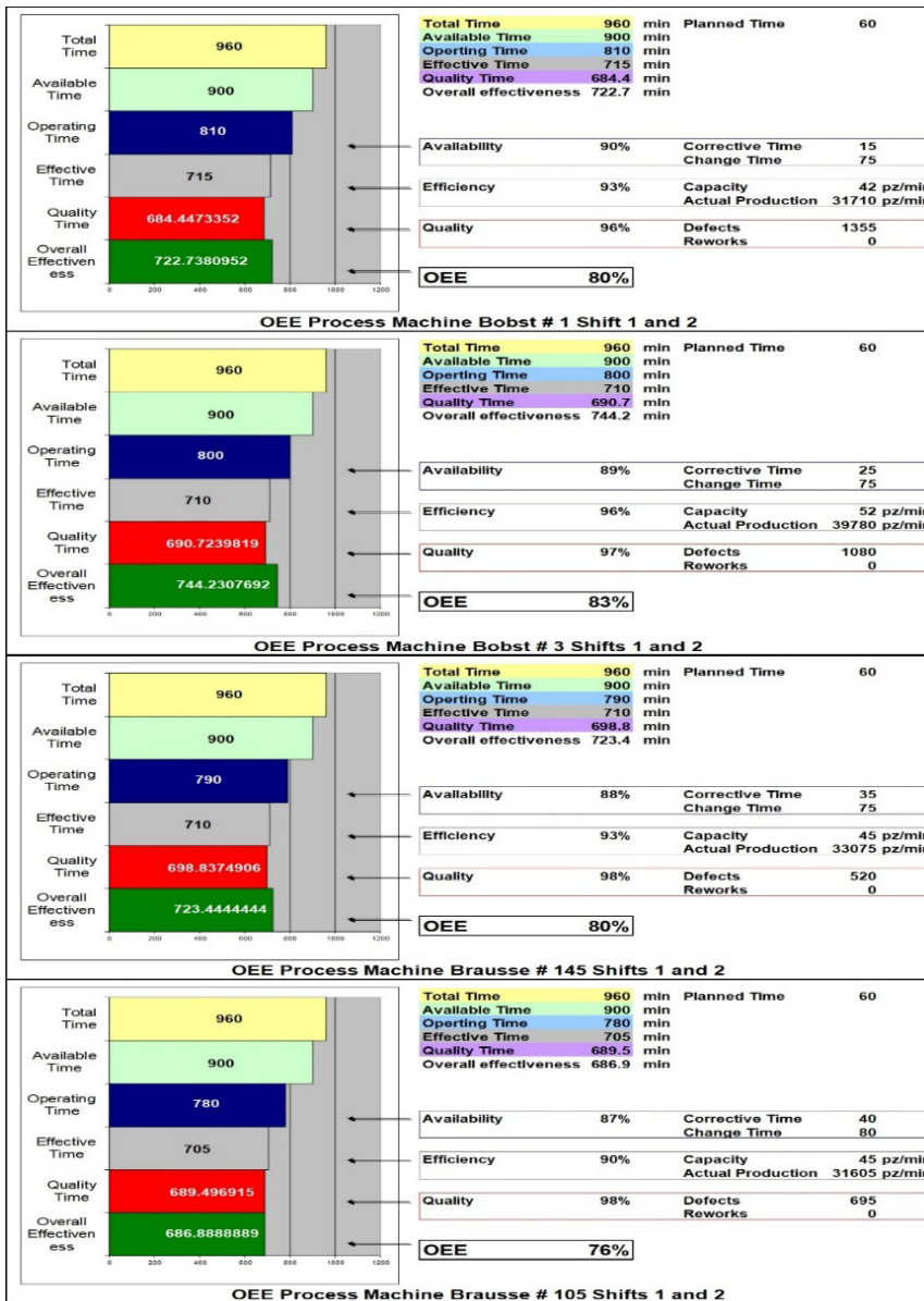
Figure 3: Calculation of the final OEE in each of the machines in two shifts
