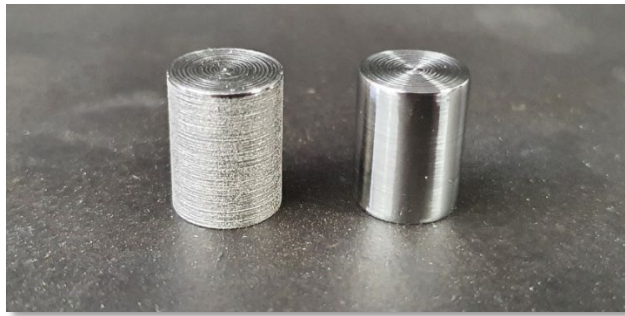
Figure 1: Sample (on the left) before and (on the right) after surface finishing
