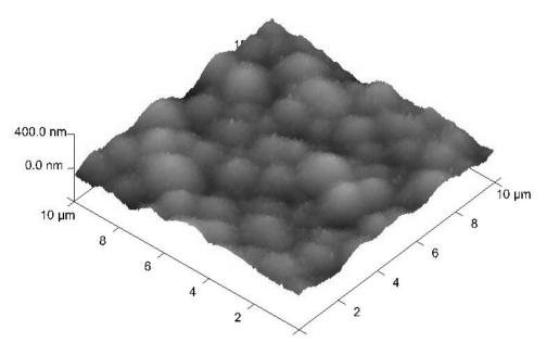
Figure 14: Atomic Force micrograph of copper deposited for 20 minutes
