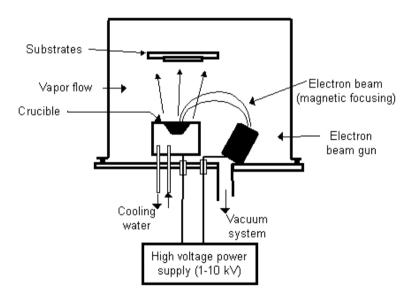
Figure 2: E-beam experimental setup
