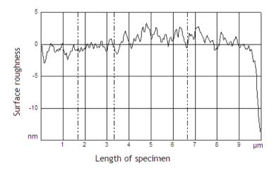
Figure 6: Atomic Force micrograph of copper deposited for 5 minutes
