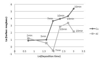
Figure 16: Log-log plot of Copper's rms surface roughness against time
