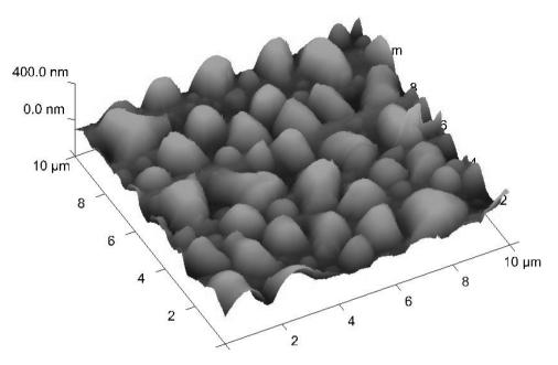
Figure 12: Atomic Force micrograph of copper deposited for 15 minutes
