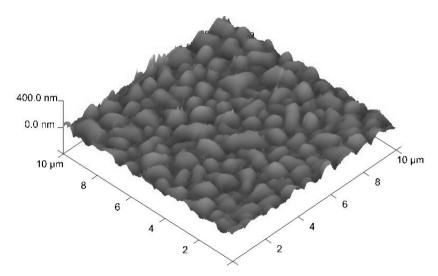
Figure 8: Atomic Force micrograph of copper deposited for 7 minutes
