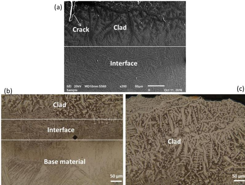
Figure 4: A typical magnified SEM micrograph and optical macrographs for all the clads: (a) clad and interface; (b) clad, interface, and base material; (c) clad
