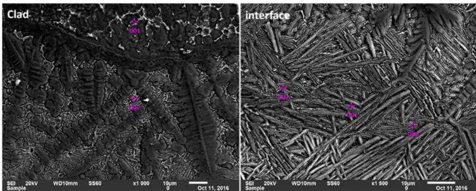
Figure 5: A typical SEM-EDS image showing how the EDS analysis was done on the clad and interface for all the clads
