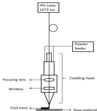
Figure 1: Schematic diagram of the laser cladding system used to clad TiAl alloy powder on Ti64 base material
