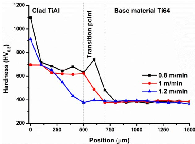
Figure 6: Microhardness graph, indicating transverse hardness of all the clads
