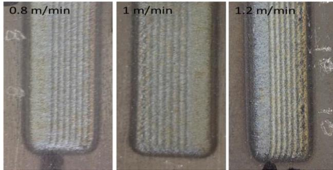
**Figure 2: Images of the as-produced clads at the different scanning speeds**
