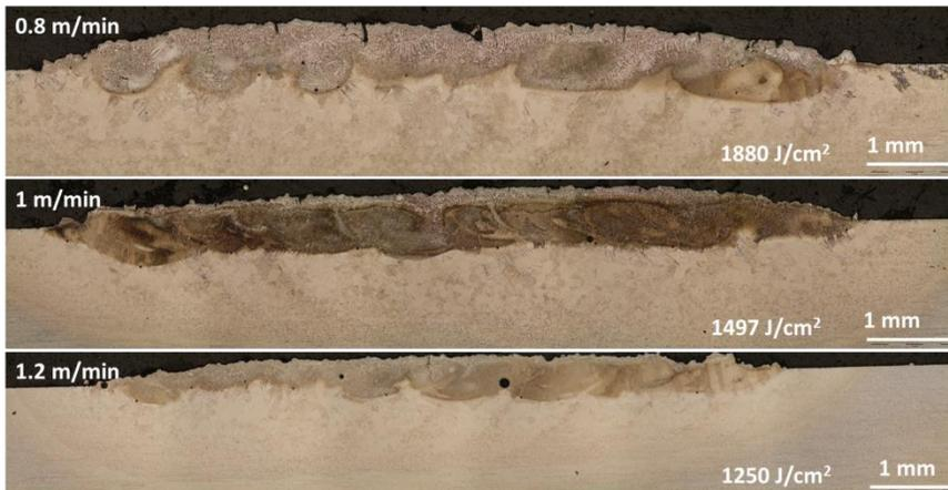
**Figure 3: Optical images of the overall image of the clads, interface, dilution, and heat-affected zone (HAZ)**
