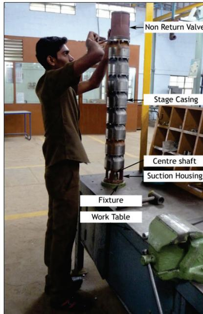
**Figure 1: Assembly of an eight-stage submersible pump**
