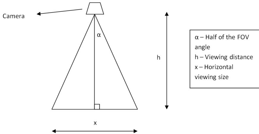
**Figure 4: Camera FOV calculation**
